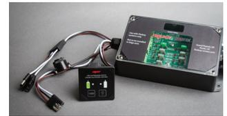
ESC Series Engine Shutdown with Helm Display
