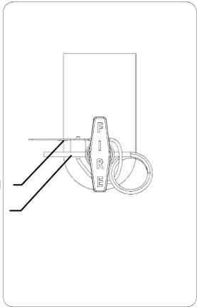
Insert Pin into Ferrule and T-Handle through holes. Wrap Tamper Seal through loop of Safety Pin and around Ferrule. Insert end of seal into side marked "ENTER" and pull tight.
