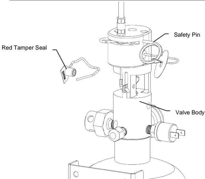
With T-Handle previously secured, remove Red Tamper Seal from Extinguisher to remove Safety Pin and store in provided hole. Cable system is now operational.
