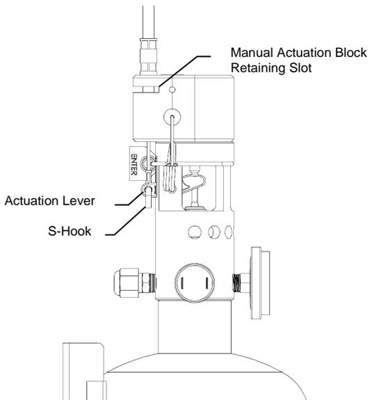
Align retaining slot of Cable with retaining slot of Manual Actuation Block.
