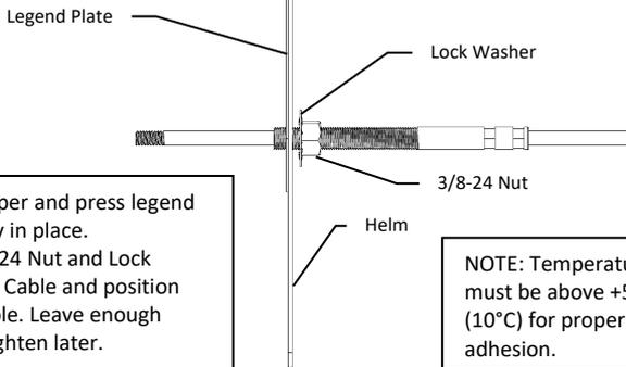
Peel off paper and press legend plate firmly in place. Install 3/8-24 Nut and Lock Washer on Cable and position through hole. Leave enough space to tighten later.
