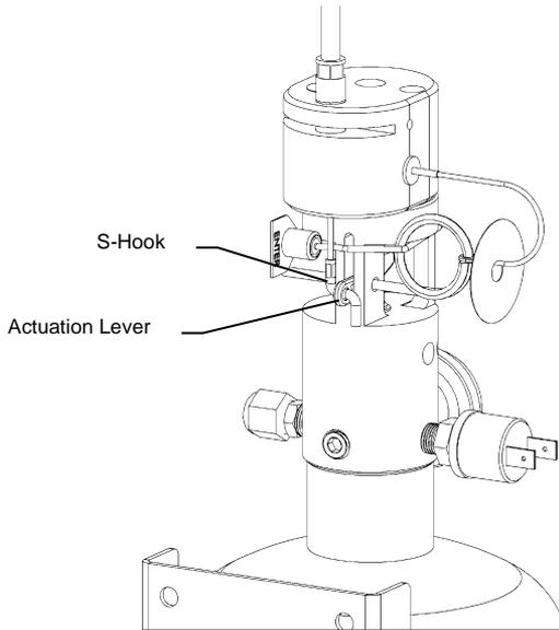
Insert S-Hook into hole of Actuation Lever.
