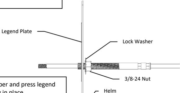
Peel off paper and press legend plate firmly in place. Install 3/8-24 Nut and Lock Washer on Cable and position through hole. Leave enough space to tighten later.
