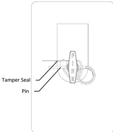
Insert Pin into Ferrule and T-Handle through holes. Wrap Tamper Seal through loop of Safety Pin and around Ferrule. Insert end of seal into side marked "ENTER" and pull tight.
