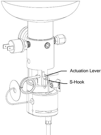
Insert S-Hook into hole of Actuation Lever.
