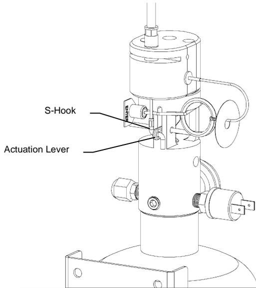
Insert S-Hook into hole of Actuation Lever.
