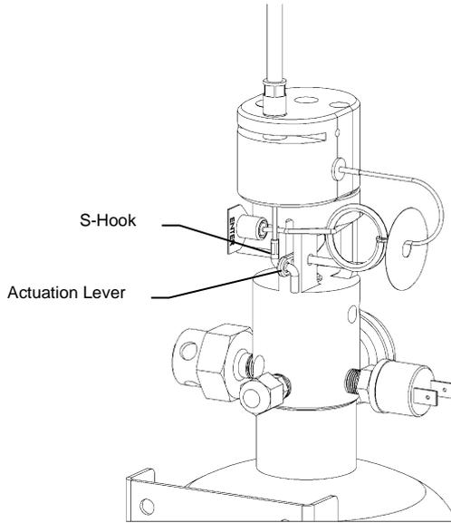
Insert S-Hook into hole of Actuation Lever.
