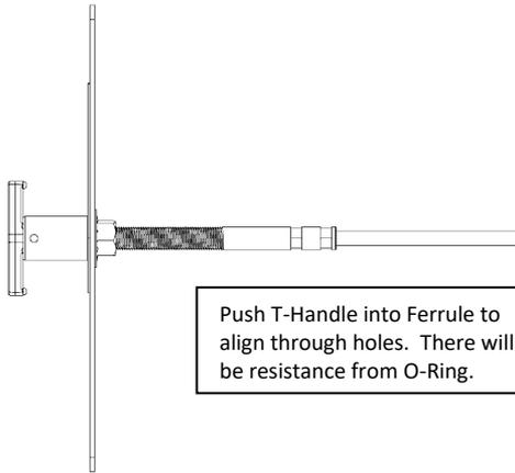
Push T-Handle into Ferrule to align through holes. There will be resistance from O-Ring.
