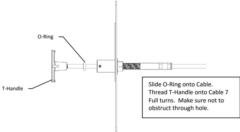
With Cable **DISCONNECTED** from extinguisher, take this time to test Cable operation. Cable should slide freely.
