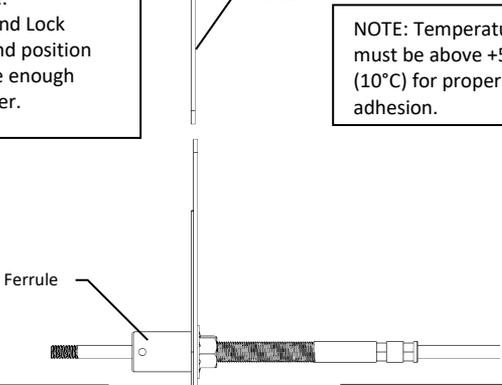
Note: Do NOT thread further than Ferrule's internal threads.
