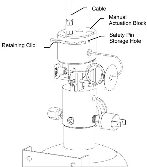
Secure Cable into Manual Actuation Block with Retaining Clip.
