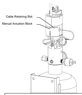
Insert extinguisher end of Cable through hole in Manual Actuation Block past retaining slot on Cable.
