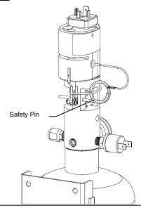
Extinguisher should be securely mounted, and Cable should be routed. Be sure the Safety Pin is in place.
