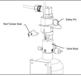
With T-Handle previously secured, remove Red Tamper Seal from Extinguisher to remove Safety Pin and store in provided hole.
