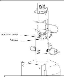
Insert S-Hook into hole of Actuation Linkage and Actuation Lever.
