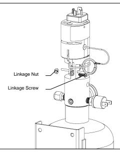
Carefully remove the Linkage Nut and Linkage Screw connecting the Actuation Linkage to the Actuation Lever.
