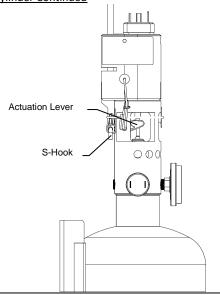
Align retaining slot of Cable with retaining slot of Manual Actuation Block.
