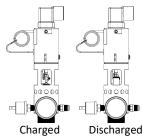
Remove and weigh the complete unit (without brackets) on a certified scale every six (6) months and record on tag provided.
