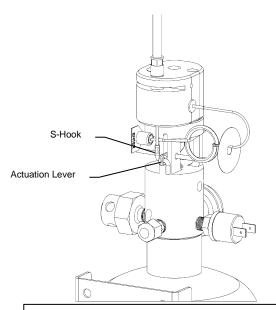
Insert S-Hook into hole of Actuation Lever.
