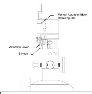
Align retaining slot of Cable with retaining slot of Manual Actuation Block.
