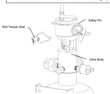
With T-Handle previously secured, remove Red Tamper Seal from Extinguisher to remove Safety Pin and store in provided hole.
